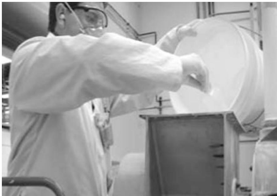
*A nanoparticle production worker wearing a personal air sampler and hearing, respiratory, and dermal protection during a pouring operation.*
